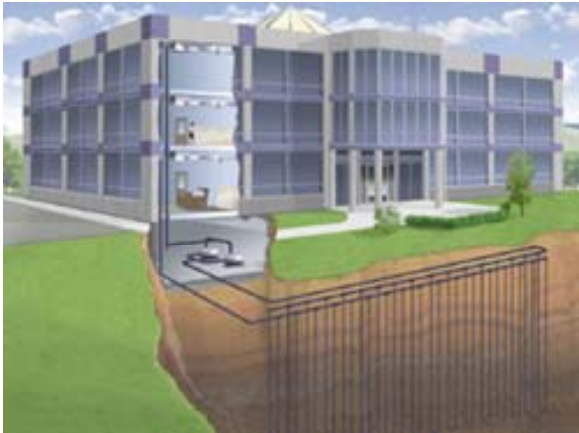
Geothermal Designs for HVAC – Closed Loop, Open Loop (Standing Column), Central Heat Pump Chiller Plant.
